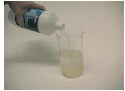
Adding demineralised water
